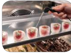
3. Sonda rilevamento temperatura Probe to survey the core temperature of the product
